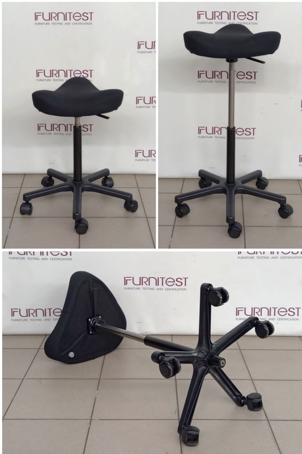
Figure 1. MOVE chair on metal cross with gas lift and wheels
